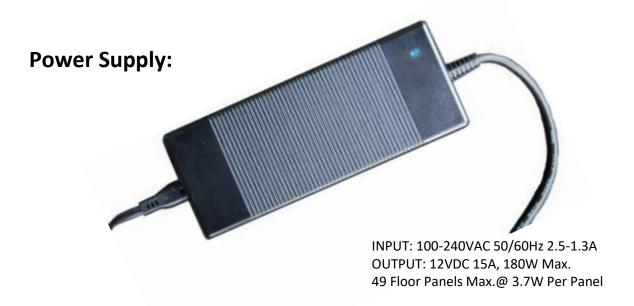
The **Power Supply** supplies all of the safe low voltage to energize your system. (**NOTE:** 49 Floor Panels Maximum) It simply plugs into any standard wall socket and connects to the **Main Power Trim** piece with a 4 pin DIN connector.
